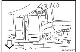
2. Remove the engine under cover. Refer to EXT-12, "Removal and Installation".
