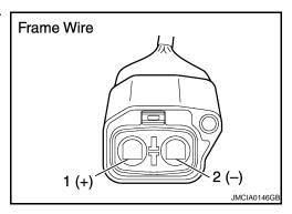
3. Disconnect the frame wire from the HV relay assembly (See HBB-105, "Removal and Installation").
