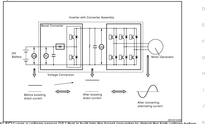
The MG ECU uses a voltage sensor (VL) that is built into the boost converter to detect the high voltage before it is boosted. It also uses a voltage sensor (VH) that is built into the inverter to detect the high voltage after it is boosted. Based on the voltage before and after it is boosted, the hybrid vehicle control ECU controls the operation of the boost converter to boost the voltage to the target voltage.
