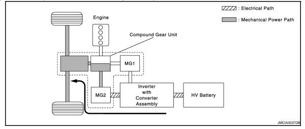
**During Acceleration with Engine**
