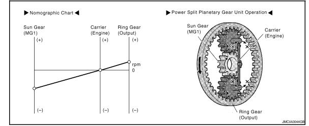
Condition of power split planetary gear unit
