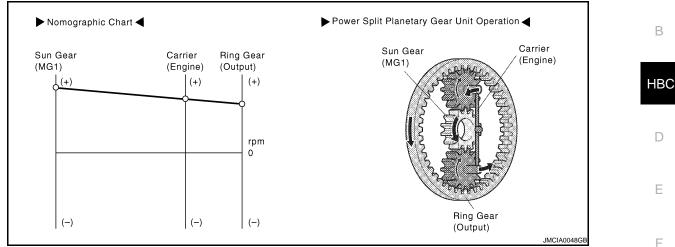
Condition of power split planetary gear unit
