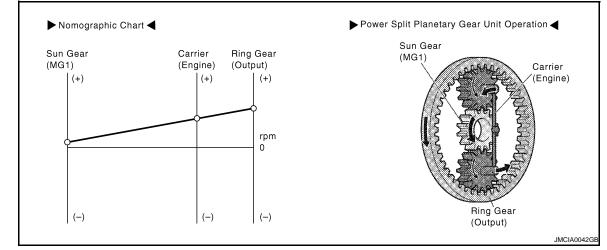
Condition of power split planetary gear unit
