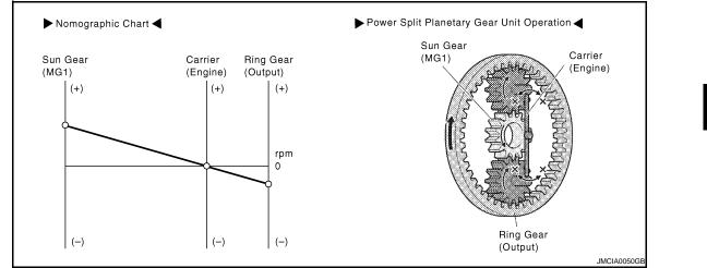
Condition of power split planetary gear unit
