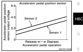
angle of the accelerator pedal from these signals, and sends the engine speed request signal and engine power request signal to the ECM. The ECM controls the throttle control motor based on these signals. Furthermore, the hybrid vehicle control ECU uses these signals for operating motor torque.
