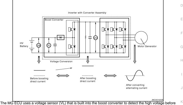
it is boosted. It also uses a voltage sensor (VH) that is built into the inverter to detect the high voltage after it is boosted. Based on the voltage before and after it is boosted, the hybrid vehicle control ECU controls the operation of the boost converter to boost the voltage to the target voltage.
