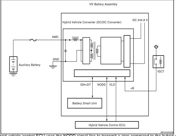
The hybrid vehicle control ECU uses the NODD signal line to transmit a stop command to the hybrid vehicle converter (DC/DC converter) and receive signals indicating the normal or abnormal condition of the 12 V charging system.
