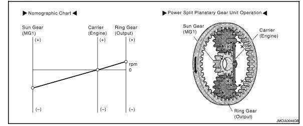
Condition of power split planetary gear unit
