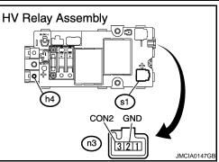
4. Measure the resistance according to the value(s) in the table below.
