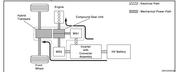
Only when driving with MG2, when the engine starts with MG1, the torque acts on the sun gear (MG1) in the (+) direction, the carrier (Engine) rotates in the (+) direction in reaction to the torque transmitted by the sun gear. The ring gear rotates in the (+) direction in reaction to the carrier rotation.
