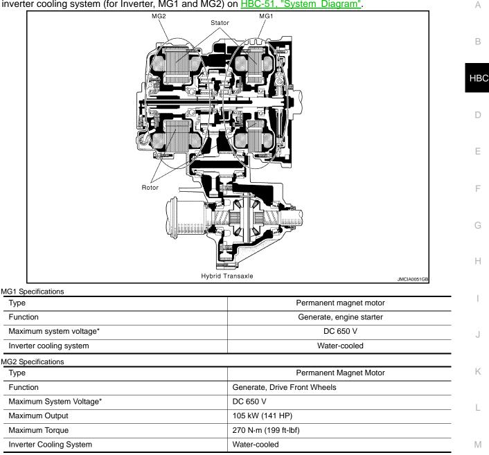
\*: These voltage are converted into an alternating current and then supplied to MG1and MG2.
