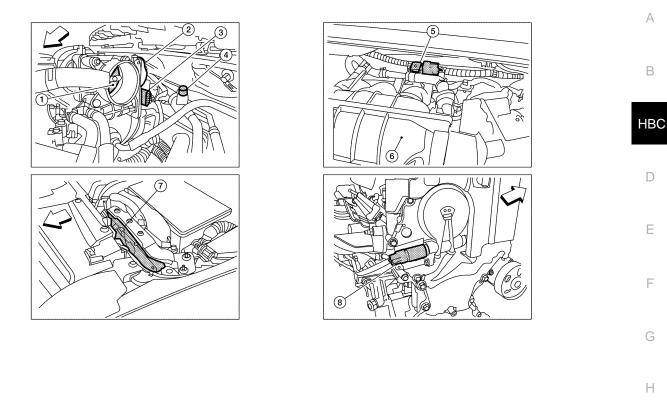
Electric throttle control actuator
