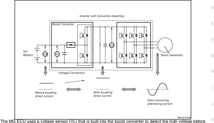
The MG ECU uses a voltage sensor (VL) that is built into the boost converter to detect the high voltage before it is boosted. It also uses a voltage sensor (VH) that is built into the inverter to detect the high voltage after it is boosted. Based on the voltage before and after it is boosted, the hybrid vehicle control ECU controls the operation of the boost converter to boost the voltage to the target voltage.
