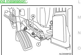
3. Remove the instrument side panel RH. Refer to <u>IP-11, "Removal and Installation"</u>.
