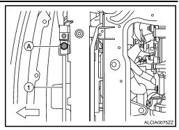
Remove the coolant drain plug (A) from the transaxle (1) and 5. Install the coolant drain plug with a new gasket to the transaxle. Coolant drain plug : 35.3 - 43.1 N·m
