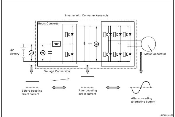
The MG ECU uses a voltage sensor (VL) that is built into the boost converter to detect the high voltage before it is boosted. It also uses a voltage sensor (VH) that is built into the inverter to detect the high voltage after it is boosted. Based on the voltage before and after it is boosted, the hybrid vehicle control ECU controls the operation of the boost converter to boost the voltage to the target voltage.
