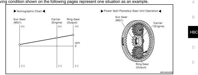
Condition of power split planetary gear unit
