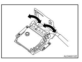
• When connecting or disconnecting pin connectors into or from the hybrid vehicle control ECU, take care not to damage pin terminals (bend or break).
