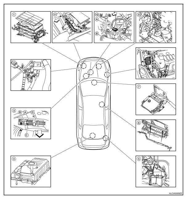
1. Inverter with converter assembly 2. Water pump with motor & bracket as- 3. sembly
