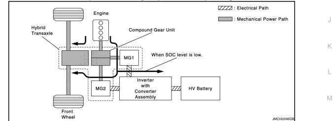
The following represents an example of the power split planetary gear unit operation under normal driving conditions. The sun gear, carrier and ring gear rotate in the (+) direction. The torque from the engine acts on the carrier (Engine) in the (+) direction, causing the sun gear and ring gear to react in the (-) direction. MG1 generates electricity by harnessing the (-) torque that acts on the sun gear.
