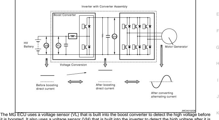
it is boosted. It also uses a voltage before and after it is boosted, the hybrid vehicle control ECU controls the operation of the boost converter to boost the voltage to the target voltage.
