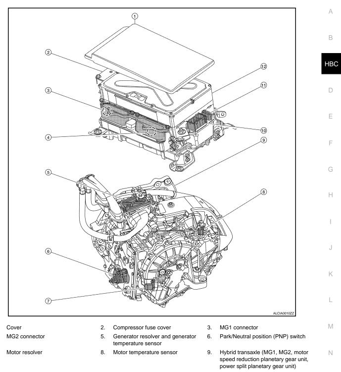
10. Inverter with converter assembly connector (MG ECU)
