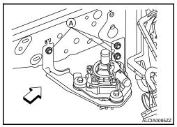
Installation Installation is in the reverse order of removal. **NOTE:** Do not use the power tool.
