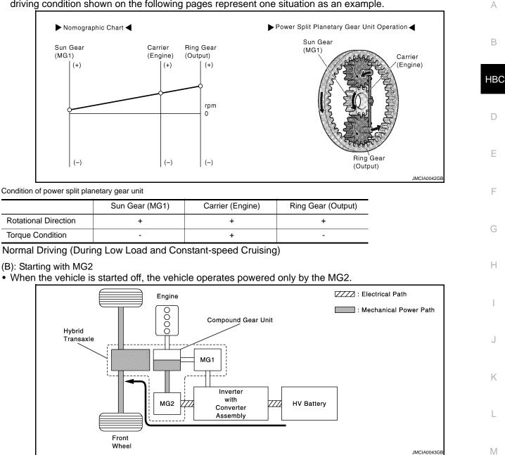
• When the vehicle starts off under normal conditions, it runs using the motive force of MG2. While driving under this condition, the rotational speed of the carrier is 0 rpm due to the engine being inactive. In addition,
