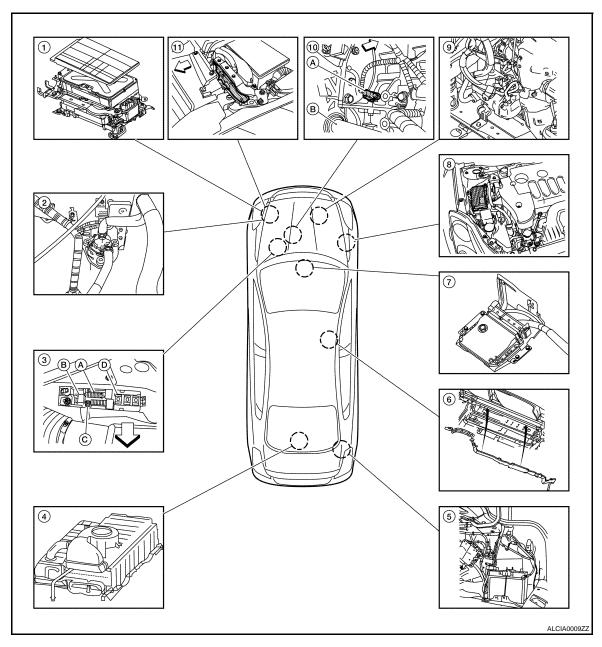
1. Inverter with converter assembly
