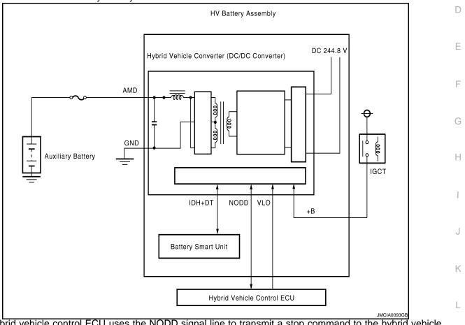
The hybrid vehicle control ECU uses the NODD signal line to transmit a stop command to the hybrid vehicle converter (DC/DC converter) and receive signals indicating the normal or abnormal condition of the 12 V charging system.
