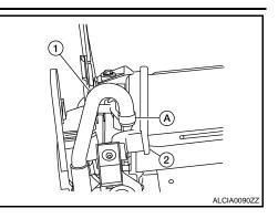
6. Remove the bolts (A), then remove the sub radiator (1) from the vehicle.
